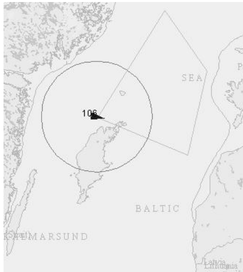
Figure 4.4: A graphical 2D map. A map application, being a federate, listening to the RTI for aircraft positions and plotting the aircrafts on a map.
