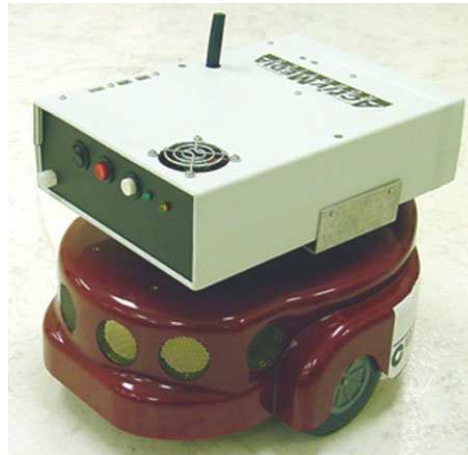
Figure 3.3: The Centibot platform. It consists of the Amigobot mobile robot, and a fairly small, on-board PC. Image was fetched from [2].
